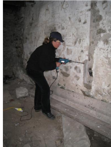
Plate 2 The Red House, Mar Lodge Estate (L, photo Coralie Mills), contains a remnant pine cruck frame from an earlier phase of building. Dendro sampling of the cruck elements (R, photo Anne Crone) has allowed them to be dated against the local Mar Lodge area woodland chronologies.
